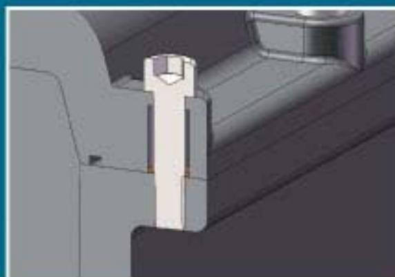
*Supermec, always paid special attention to on-site installation issues. Introducing new EJB A series, we designed a special anti-loosening bolt to make the job easier for maintenance staff.*
